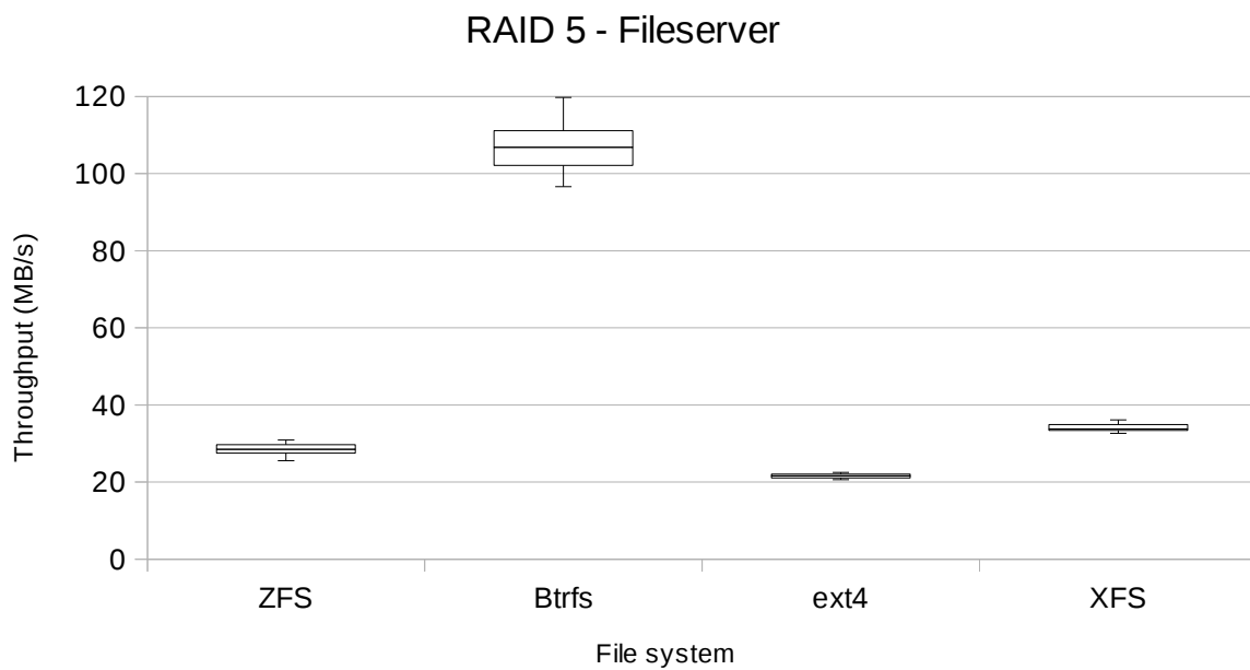
Figure 8: Filebench Fileserver experiment with RAID 5 setup.
