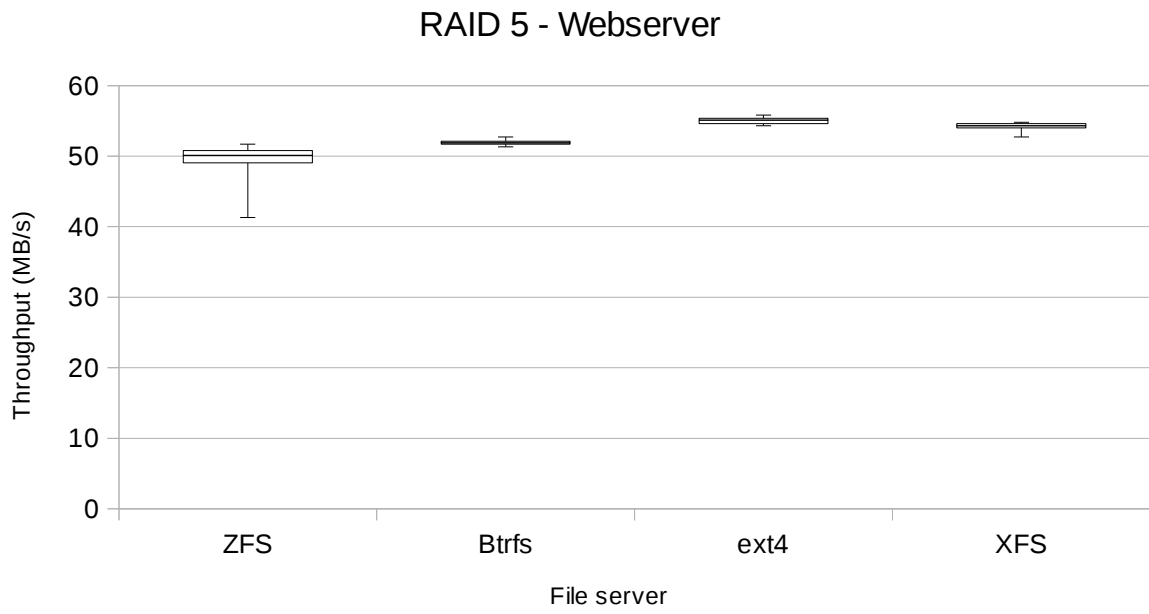
Figure 32: Filebench Webserver experiment with RAID 5 setup.
