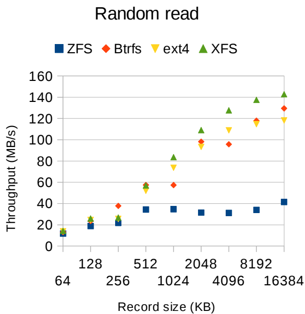
Figure 12: IOzone random read result for single disk. Figure 13: IOzone strided read result for single disk.
