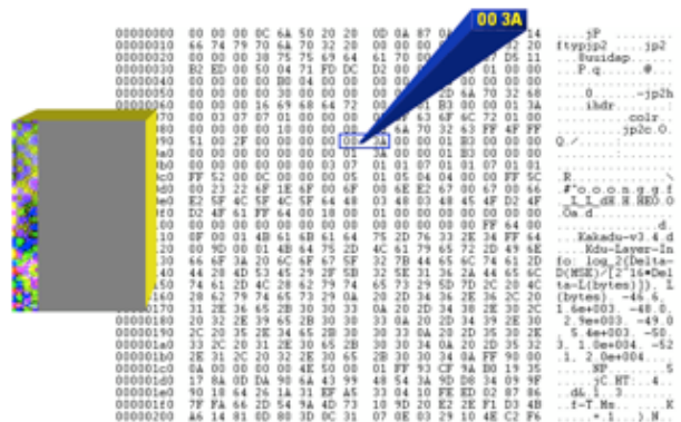
Figure 8b - Impact on the image of corrupted header height values
