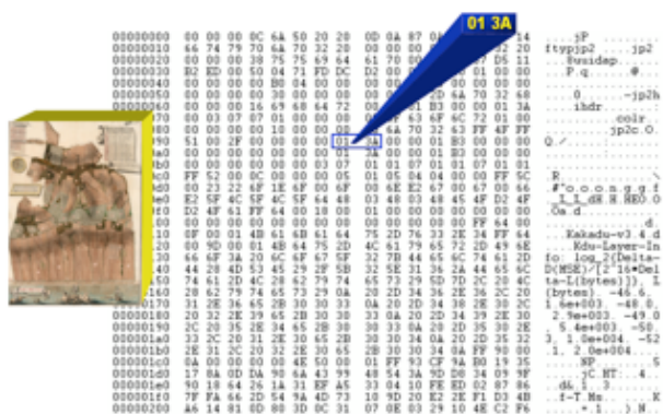
Figure 8a - JP2000 header: highlighted values represent image height
